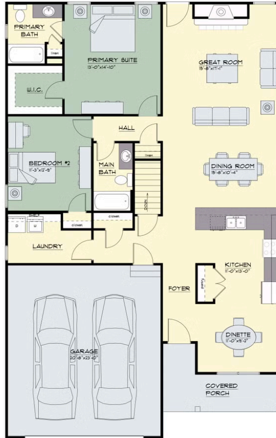
FLOOR PLAN THE "ANGELINA 225" 2/3/2025 LIVING AREA: 1550 S.F. OVERALL DIMENSIONS: 31'-4" x 59'-0"
