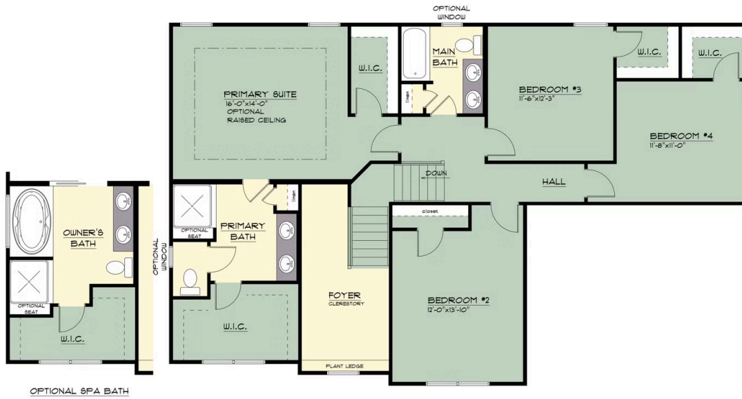
SECOND FLOOR PLAN THE "HAWTHORNE 22A" 4/4/2025 LIVING AREA: 1265 S.F. CLERESTORY 133 S.F. TOTAL AREA 1398 S.F.
